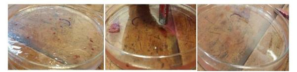
Figure 4: Extraction of lubricant oil from oil-water mixture using iron oxide nanoparticles
