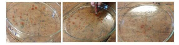
Figure 3: Extraction of mustard oil from oil-water mixture using iron oxide nanoparticles
